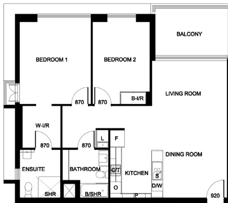
Figure 107: Apartment floor plan — Adaptable after adaptation
