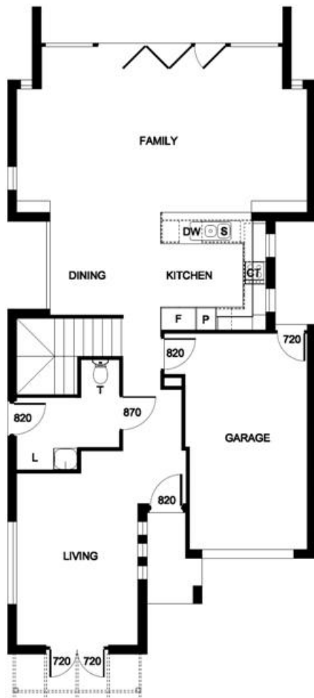
Figure 92: Separate house — Visitable floor plan
