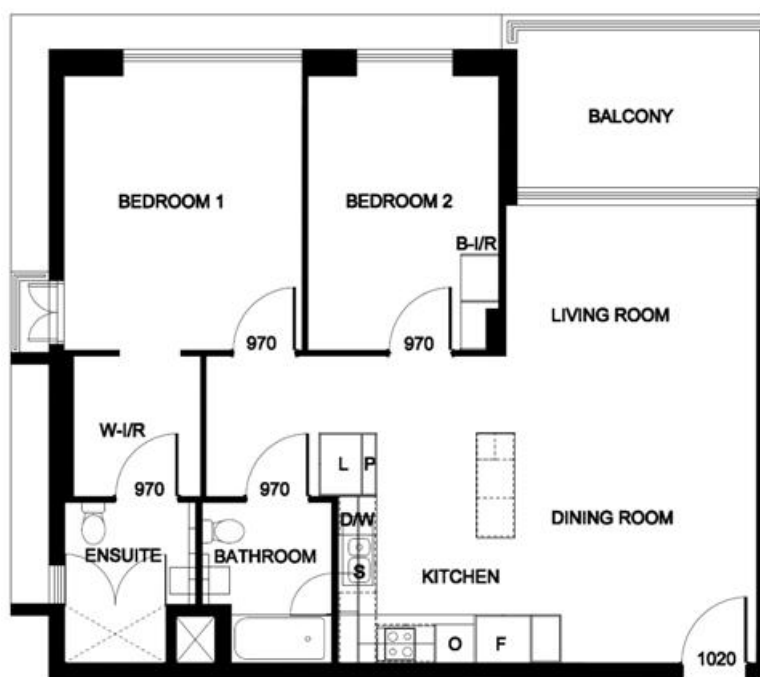
Figure 108: Apartment floor plan — Universal
